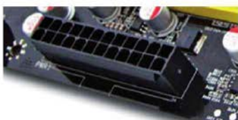
↑ Conector de corriente ATX12V 24p.
