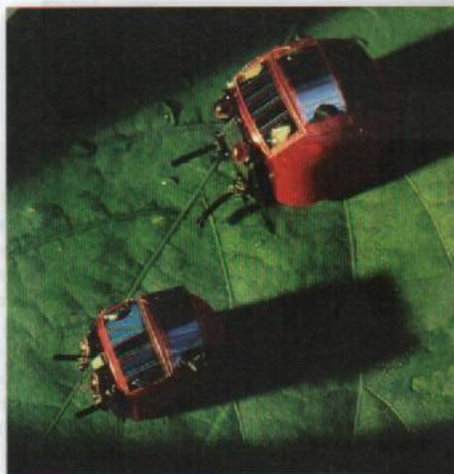
Ladybug robots crawl down a leaf. The robots are powered by solar power collectors attached to their backs.
