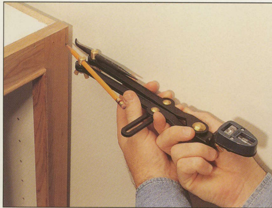
A transfer scribe accurately follows the contours of a wall and draws a matching line onto a scribe rail. Once the rail is planed or sanded to this line, the cabinet will fit seamlessly when it is installed.
