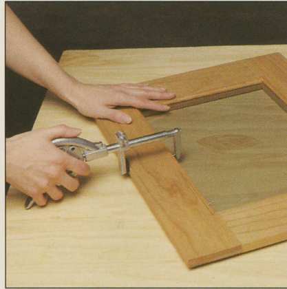
A brad driver secures a strip of molding to the frame of a kitchen cabinet door, sandwiching a central pane of glass between the molding and a rabbet cut into the inside edge of the frame. For more on building glass doors, see page 69.
